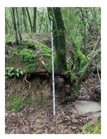
**Photo 3.** Close-up of trunk of bay tree depicted in Photo 2 above. As seen on the stadia rod, the top of bank exceeds 4 ft.
