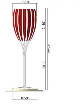
SITE SCULPTURE: 32' TALL WINE GLASS CONSTRUCTED FROM 16 x 2" x 2" SQUARE TUBE STEEL FRAMES, PAINTED WHITE (P5), EACH COLD FORMED TO WINE GLASS PROFILE, WELDED TOGETHER AND FACED WITH RED TRANSLUCENT POLYCARBONATE PANELS (TP1 SEE SHEET A04.1 & COLOR BOARD). SCULPTURE SITS ATOP A MULTI-LEVELED 27'-6" DIAMETER CIRCULAR CONCRETE BASE OF BEIGE AND TERRA COTTA PIGMENTED CONCRETE.
