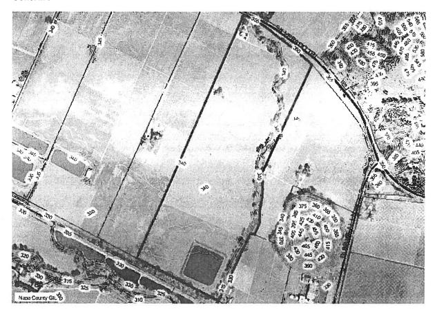
This map shows elevation contour lines. Within the Napa River Watershed, roughly the western half of the county, the contour interval is 5 feet. The rest of the county has a 10 foot contour interval. This elevation information was derived during the 2002 Orthophoto Project. Changes to the land surface that occured after April 20, 2002 will not be reflected in these contour lines.
