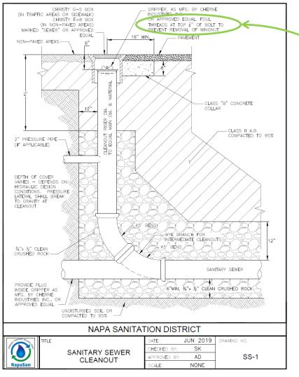
REQUIRE FOULING OF THREADS TO PREVENT REMOVAL OF WINGNUT
