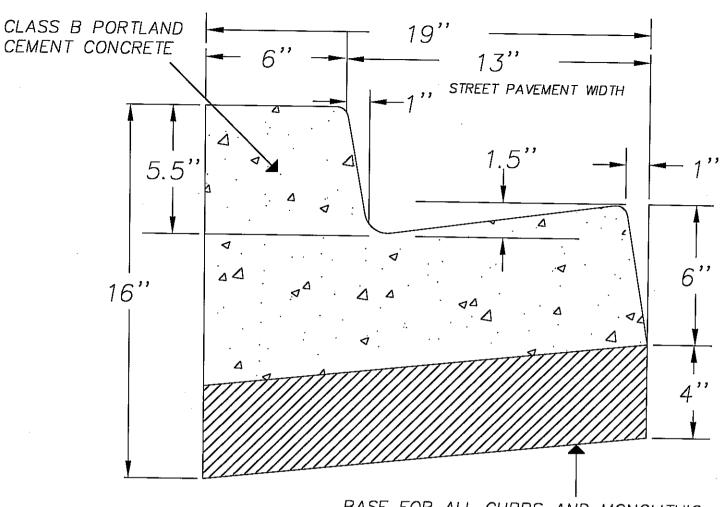
BASE FOR ALL CURBS AND MONOLITHIC CURB AND GUTTERS SHALL BE CLASS 2 AGGREGATE BASE OR APPROVED CLEAN GRANULAR MATERIAL, MIN. SAND EQUIVALENT OF 30.
