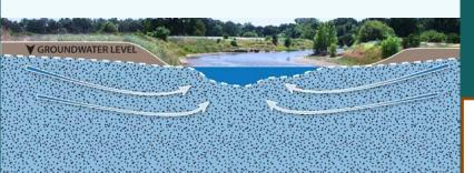
Groundwater Pumping Stream Loses Water/ Recharge to GW
