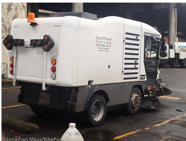
The RAVO sweeper is 105-inches tall, 89-inches wide (7.4 feet), and 178-inches long.
