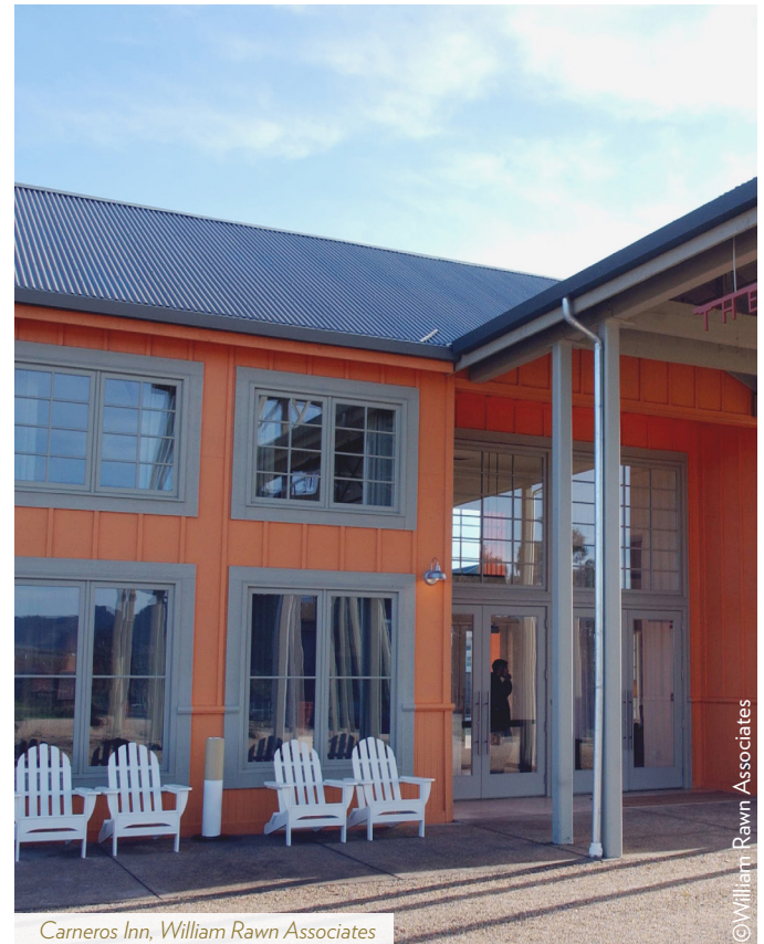
Figure B.3.1g Gable-roofed building masses reference farm structures. Contemporary materials with the pronounced vertical grain reference corrugated metal and board and batten of farm vernacular. Deep recesses that cut into the building mass relate to function and create additional contemporary character.
