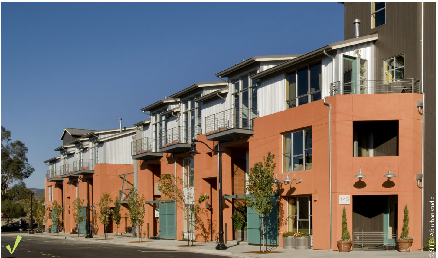
Figure 4.1.3g Material and Façade Composition. Good (top left): Change of color or material at the ground level reinforces the human scale. Good (bottom): Articulation reflects interior spaces. Material change supports street level definition. Bad (top right): All one material. Color change is not associated with articulation and bisects upper story windows.
