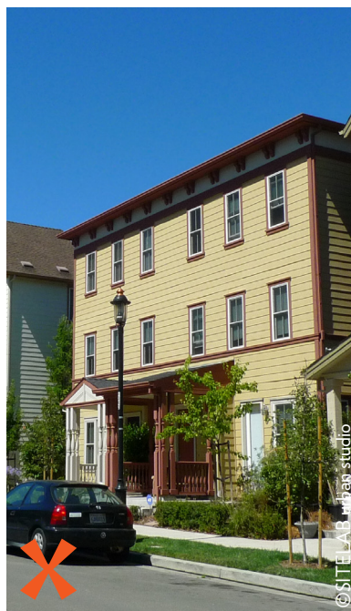
Figure 4.1.6c Building Walls. Good (left): Walls have perceivable thickness with window reveals, projections, deep recesses, and overhangs. Bad (middle, right): Building walls are planar and have poor thickness and visual character due to lack of window reveal and insufficient depth of articulation.
