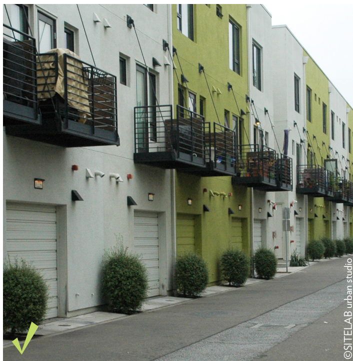
Figure 4.1.6l Garage Door Sequence. Good (left): Recessed garage doors create depth. Single doors ensure planting opportunities. Alternating colors adds variety to the rear building wall. Bad (right): Minimal depth of the garage door recess creates a flat façade. Wide garage doors limit opportunity for planting.
