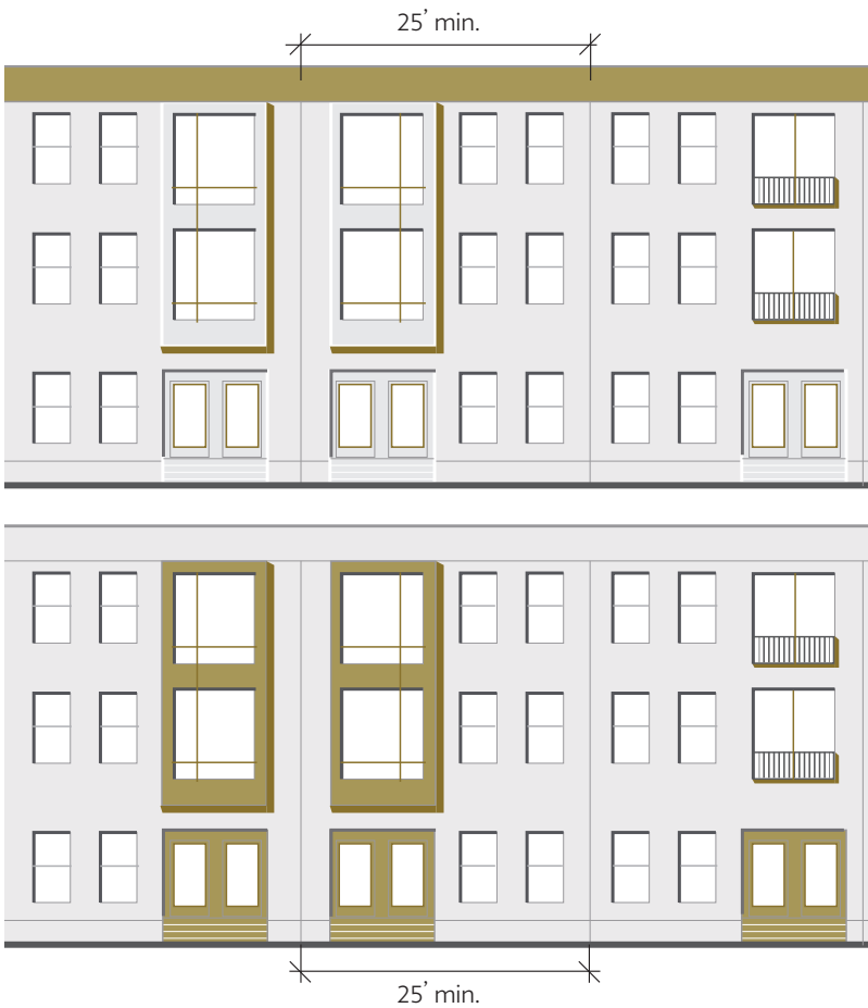
Figure 4.2.6g Articulate building façades a minimum of every 25'. Façade modulation should have vertical rhythm. Accent with reveals, recesses, entries, details, and projections.
