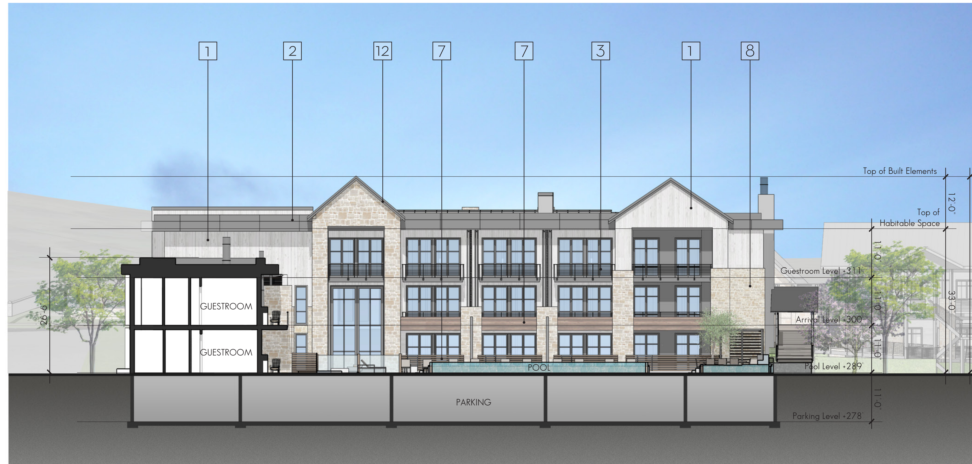
COURTYARD SECTION-SOUTH ELEVATION
