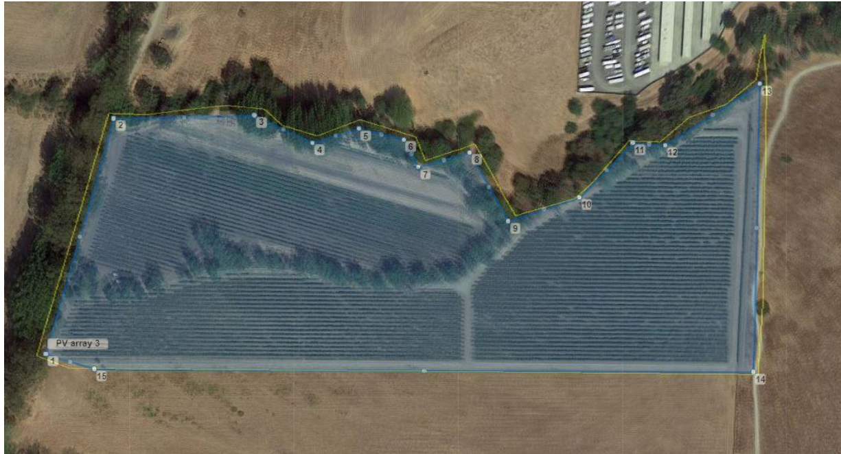
Figure 2. Soscol Ferry Solar PV Array in ForgeSolar (blue area with numbered vertices) with Overlay of the Parcel Outline (yellow line) of the Entire Parcel on which the Soscol Ferry Solar Site is Located
