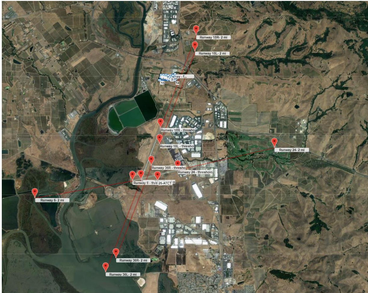
Figure 5. Approach Flight Paths (Red Lines) to Napa County Airport’s Six Runways and Air Traffic Control Tower (“25 – ATCT” just south of the center of runway 6/24) as Modeled in ForgeSolar
