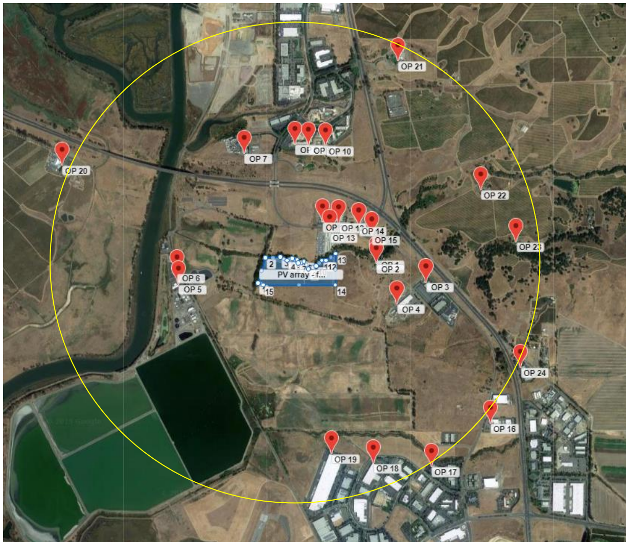
Figure 12. Building Observation Points (OP 1 to OP 24) at Residential and Commercial/Industrial Buildings within 1 Mile Radius (Yellow Circle) of the Center of the Proposed Solar Facility as Modeled in ForgeSolar
