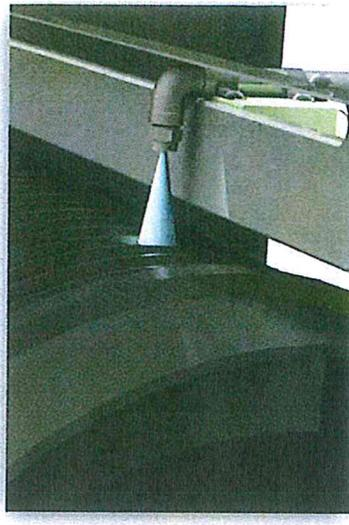
1000psi – 1.8GPM Spray Nozzle continuously travels length of screen for ultra effective cleaning using much less water than conventional spray bars
