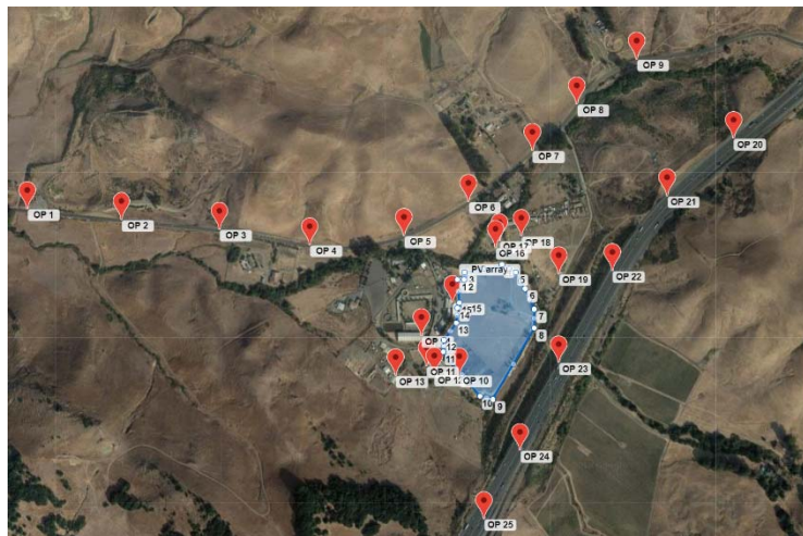
Observation Points Analyzed in ForgeSolar, in Addition to the Flight Paths at Napa County Airport (Not Shown, approximately 4 miles to the NW); OP1 to OP9 on American Canyon Road and OP20 to OP25 on Interstate-80
