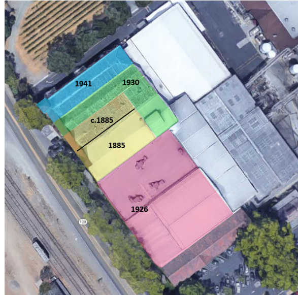
Figure 2. Construction chronology (ARG). Note: the 1885 building appears to have been completed in two sections, but research did not identify a concrete date of construction beyond 1885.
