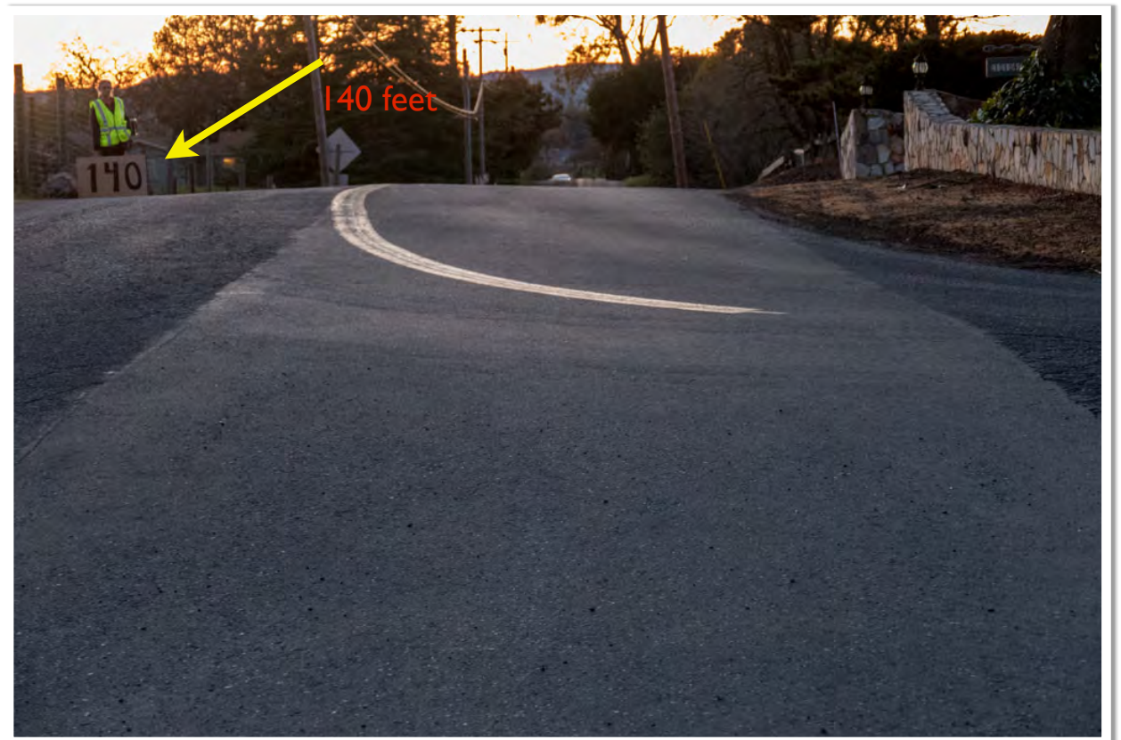
Visible Line of Sight is 140 feet from the Kreuzer Lane stop sign (at stop line). In image above, a car can be seen in the far distance, but will shortly disappear into the dip in the road and then reappear at 140 feet.
