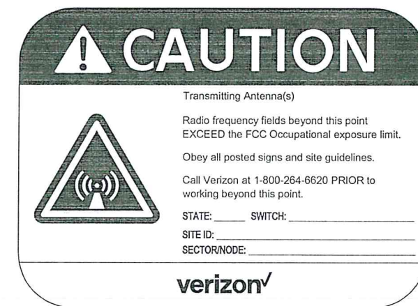
3 VERIZON WIRELESS TYPICAL CAUTION SIGN
