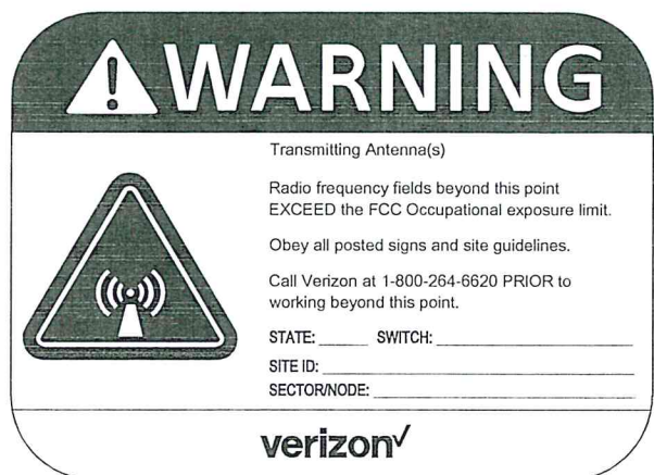
4 VERIZON WIRELESS TYPICAL WARNING SIGN
