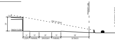
TYPICAL EQUIPMENT SCREEN LINE OF SIGHT SCALE: 1/4" = 1'-0" NOTE: LINE OF SIGHT TAKEN FROM 6'-0" ABOVE FINISH GRADE
