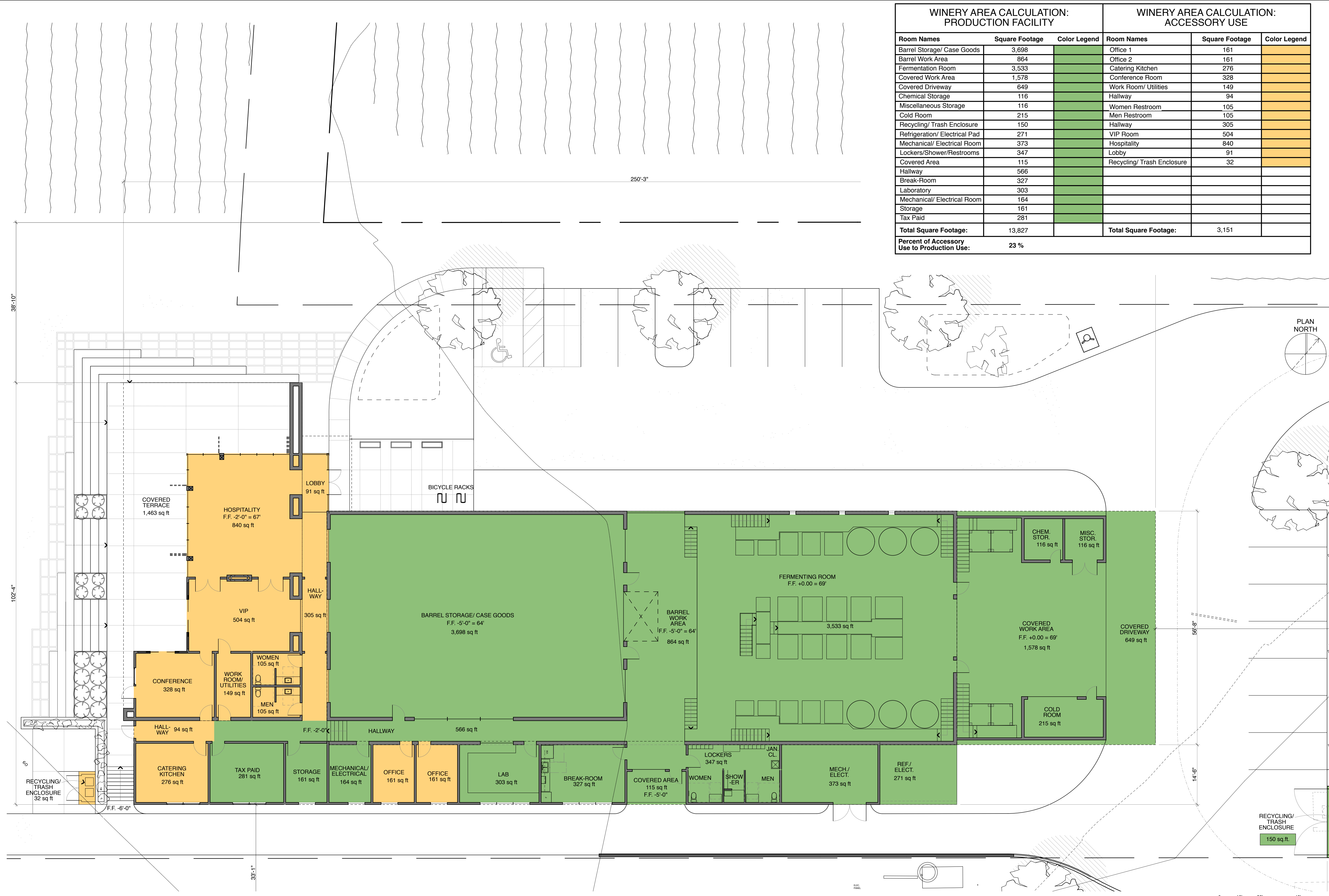
1 WINERY PRODUCTION AREA & ACCESSORY AREA PLAN SCALE: 1" = 10'
