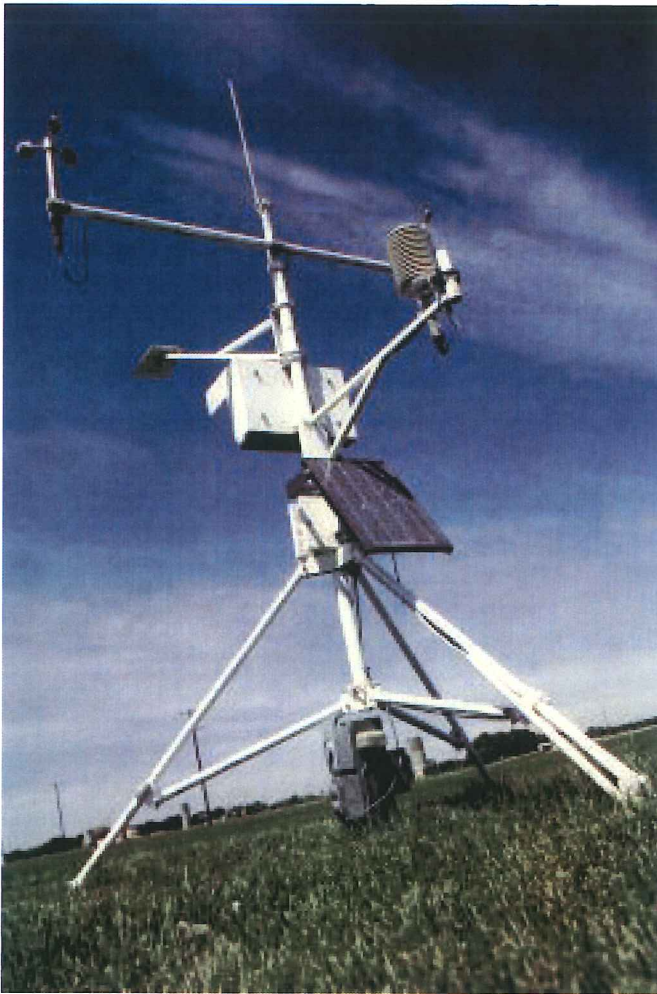
A specialized weather station (CIMIS station) or a Class A evaporation pan (background) can be used to determine reference evapotranspiration (ET 0 ) for a site. Daily CIMIS data is available online at www.cimis.water.ca.gov .
