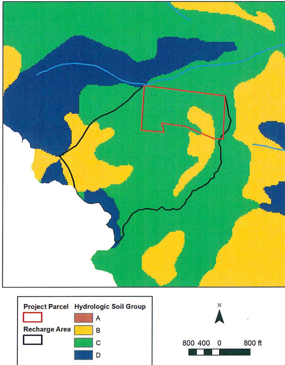
Figure 6: Soils map used in the SWB model.
