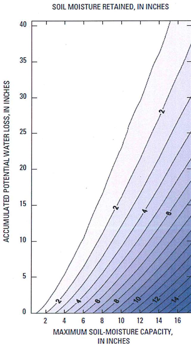
**Figure 4: Soil-moisture-retention table (Thorntwaite and Mather, 1957).**
