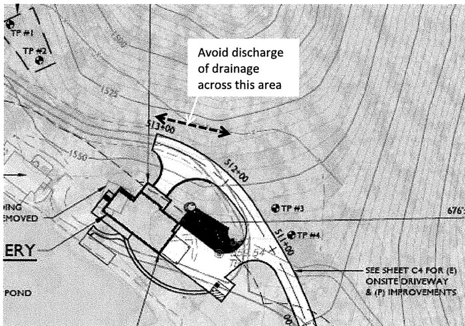
Figure 3. Recommended drainage management at winery site.
