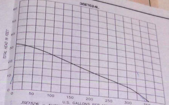
3SE1524L U.S. GALLONS PER MINUTE 3SE1524L - AUTOMATIC & MANUAL - DISCHARGE - 3" - HP 1.5 CRANE MODEL NO. 3SE1524L
