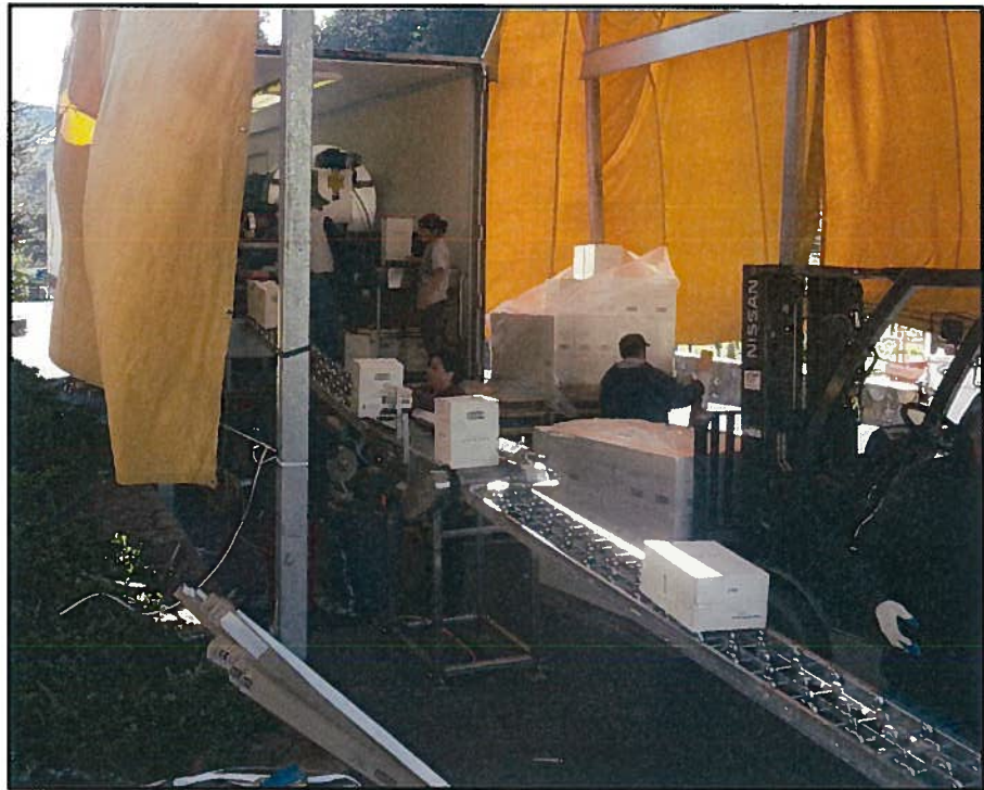
Figure 3: Detail of Rear (open) Face of Bottling Truck
