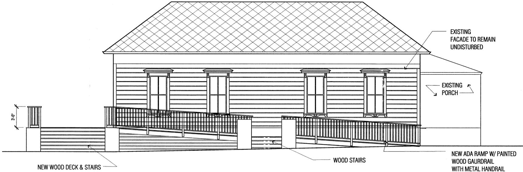
BLDG - B SOUTH EXTERIOR ELEVATION
