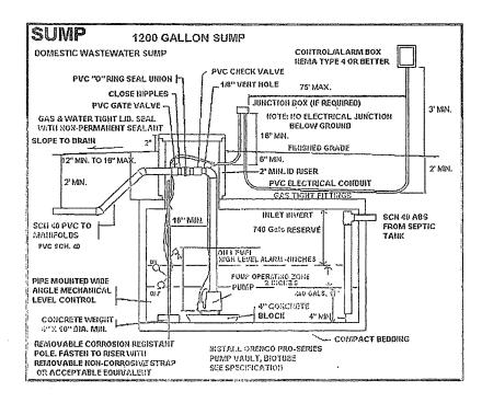
All tanks will have Orenco 24 inch diameter risers over the manholes, brought to grade. All tanks will be thorosealed so as to be watertight.
