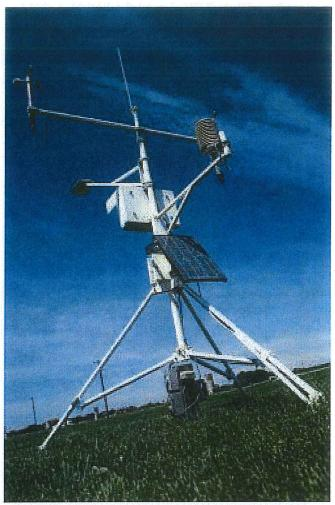
A specialized weather station (CIMIS station) or a Class A evaporation pan (background) can be used to determine reference evapotranspiration (ET<sub>o</sub>) for a site. Daily CIMIS data is available online at www.cimis. water.ca.gov.
