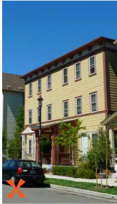
Figure 5.15 Bad: Building walls are too planar and have poor thickness and visual character due to insufficient window reveal and insufficient depth of articulation.
