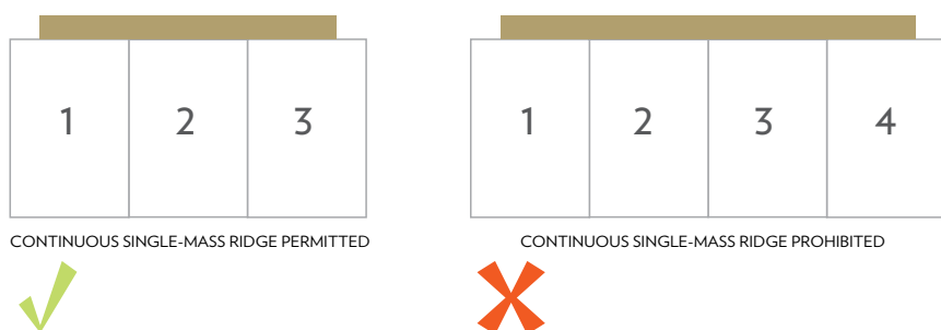
Figure 5.12 Single roof mass with continuous ridge line permitted on maximum of 3 consecutive townhouses.
