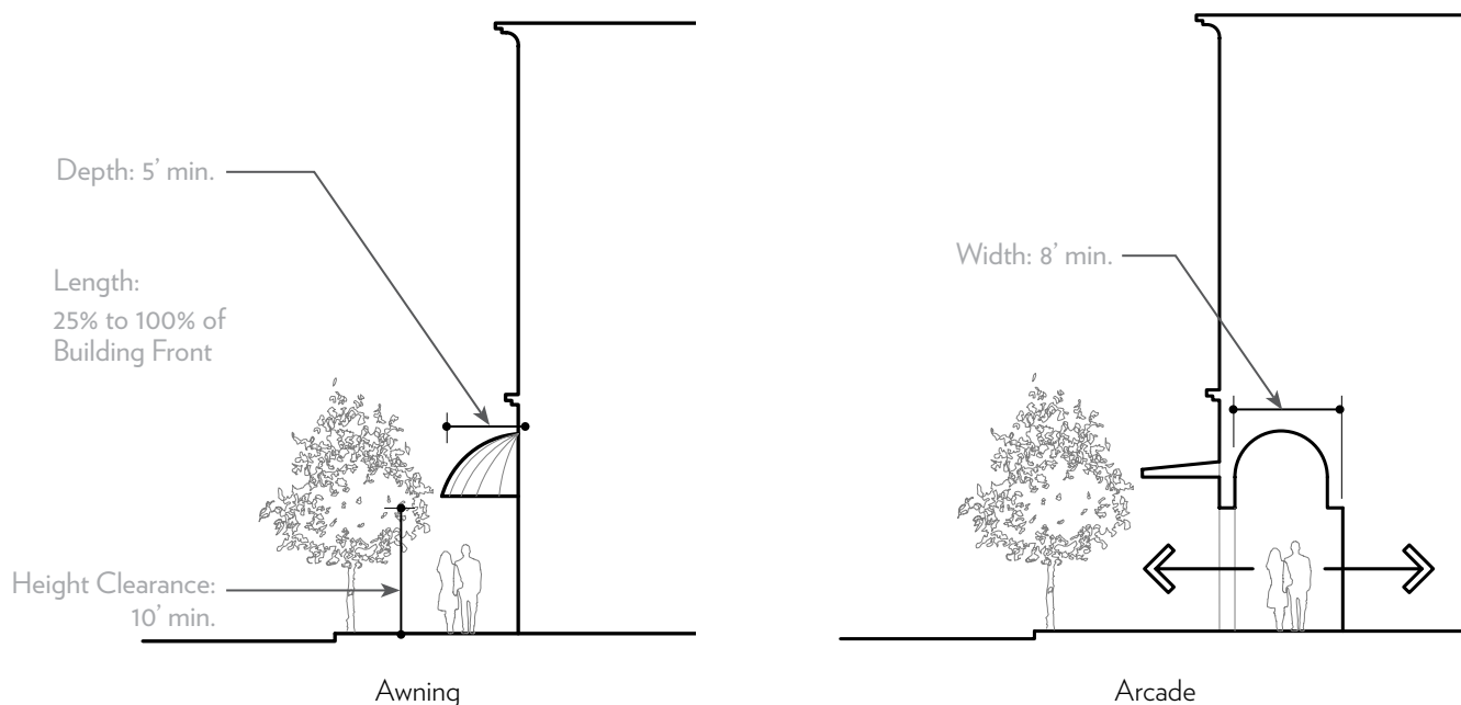
Figure 5.27 Typical Awning Section. Awnings and marquees that are forward of setback are recommended. Arcades are permitted.
