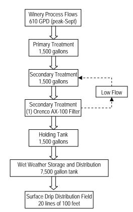
Figure 2: Proposed Process Wastewater Treatment System Schematic
