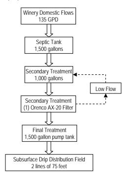
Figure 1: Proposed Domestic Wastewater Treatment System
