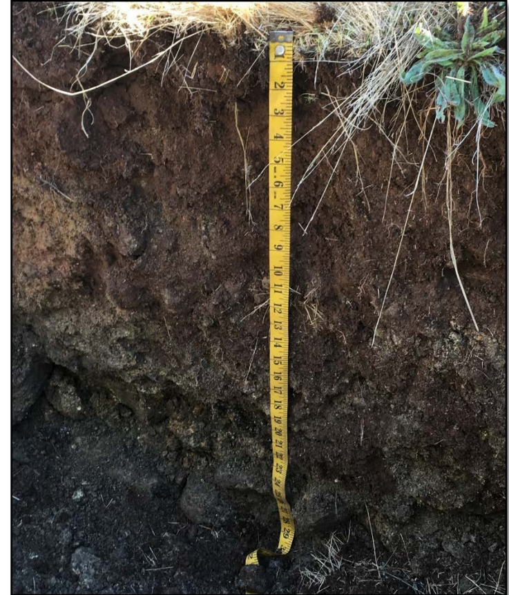
Soils Post-Ripping and Blasting – 22 inches deep
